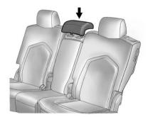
The center seating position has an integrated headrest that can be adjusted the same way as the head restraints.
